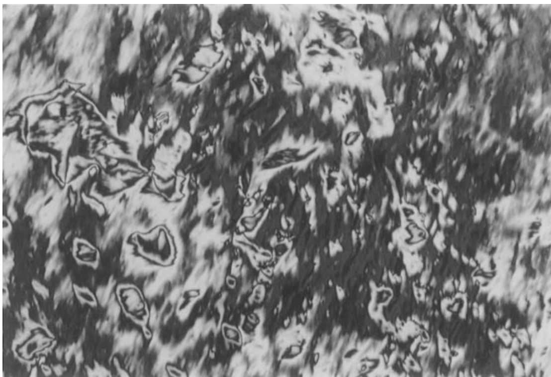
Figure 1. Schlieren texture shown by the Sc phase of \text{Cu}[\text{L}_2(14)] at 215 °C.
